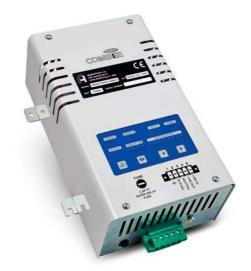
After setting the parameters, the regulator operates automatically without the need for further actions. The COMBI regulator can be installed in single and three phase electrical systems, either in cabinets or wall while maintaining an IP20 protection degree.
